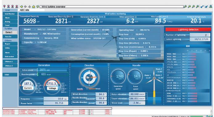
Example display of wind turbine monitoring
